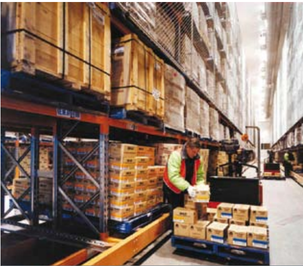
Pallet Live Storage First-in first-out automatic stock rotation
