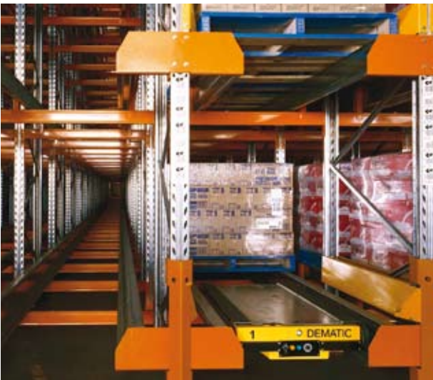
Pallet Runner System Maximum storage and operational effectiveness
