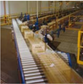
Accumulation & transportation conveyors
